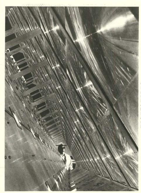
CONCENTRATED sunshine is viewed by Gene Hammons (5132) in this system that includes 135 plastic Fresnel lenses (right) focusing upon an equal number of silicon solar cells at left. Electrical output of cells is increased about 50 times using concentrated light.
